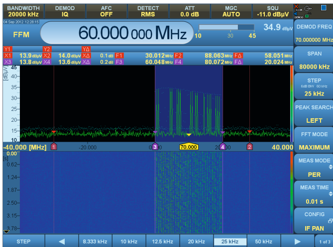
Signal sequence of a frequency hopping radio: 2000 hops per second and 20 MHz hop bandwidth (coverage of the complete tactical band from 30 MHz to 88 MHz possible).
